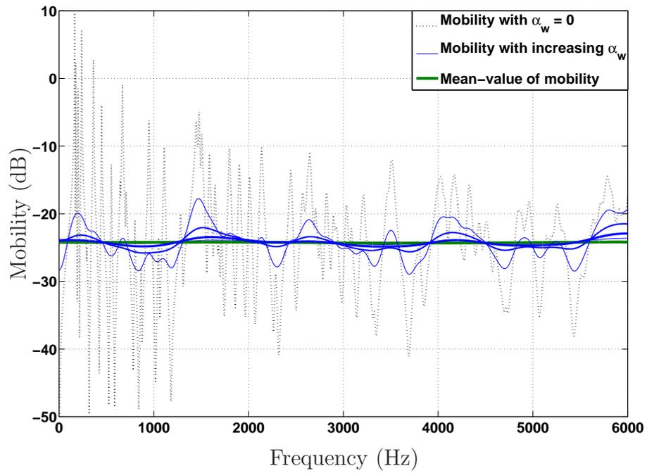
Figure 4: Mobility of a simulated plate with different values of the damping parameter  $\alpha_w$ . When  $\alpha_w$  is large enough, the mobility is then a straight line, corresponding to the mean-value of mobility.
