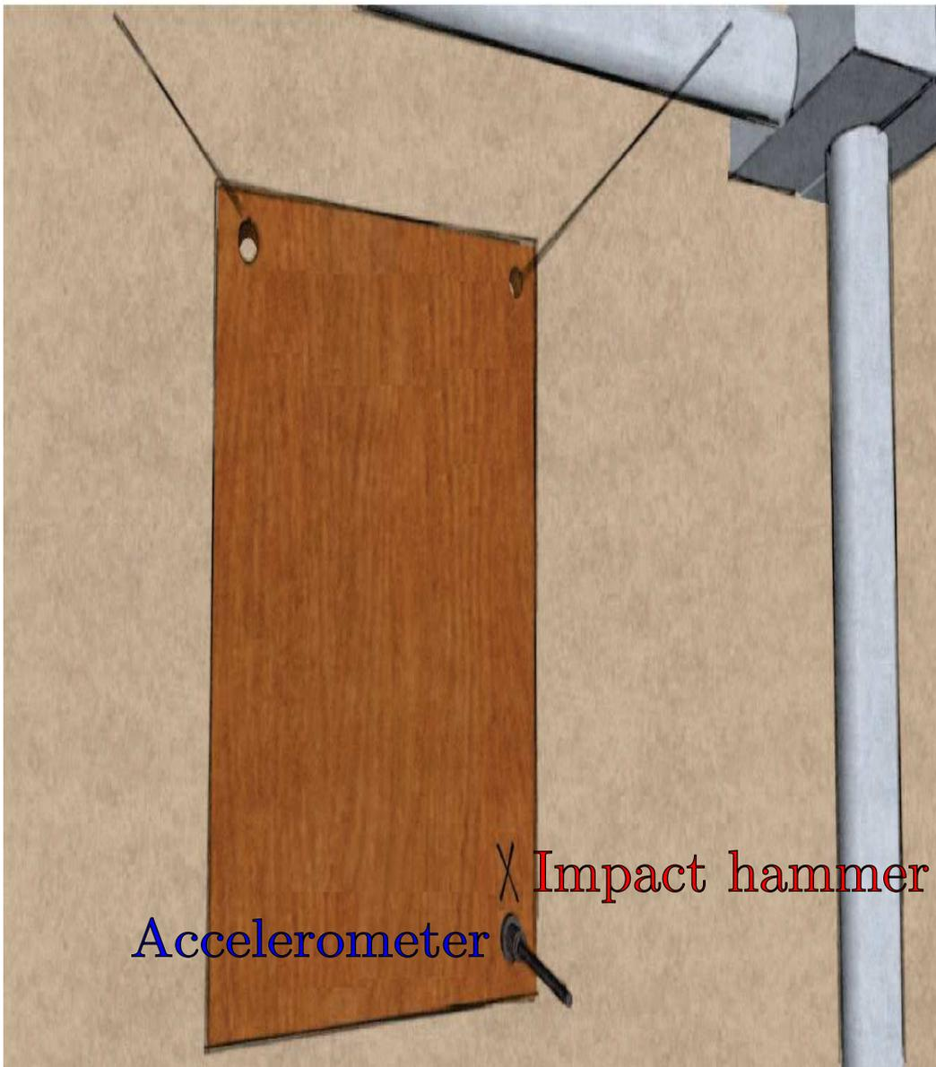
Figure 9: Experimental setup for panel mobility measurement.
