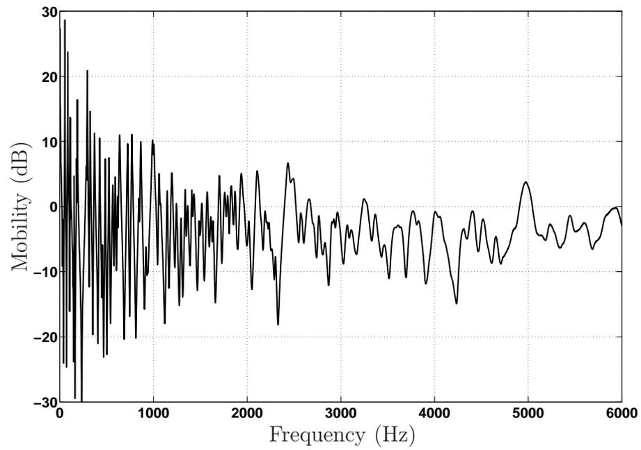
Figure 2: Driving-point mobility of the  $500 \times 190 \times 2$  mm spruce panel. The reference at 0 dB corresponds to a mobility of  $0.094 \text{ m}\cdot\text{s}^{-1}/\text{N}$ , namely the mobility of a 2mm-thick finite panel having the typical mechanical properties of spruce.
