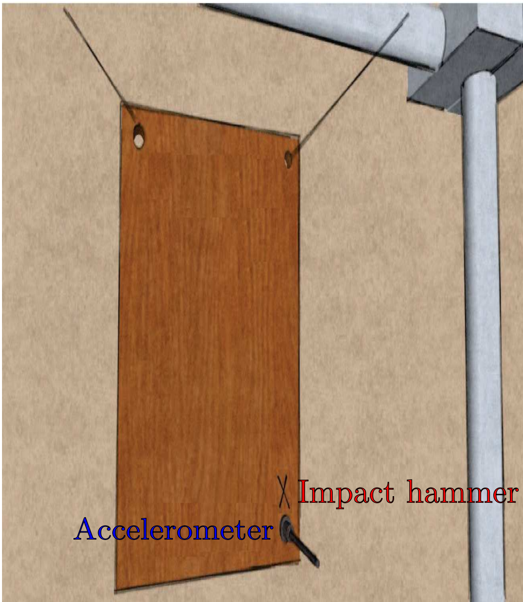
Figure 9: Experimental setup for panel mobility measurement.
