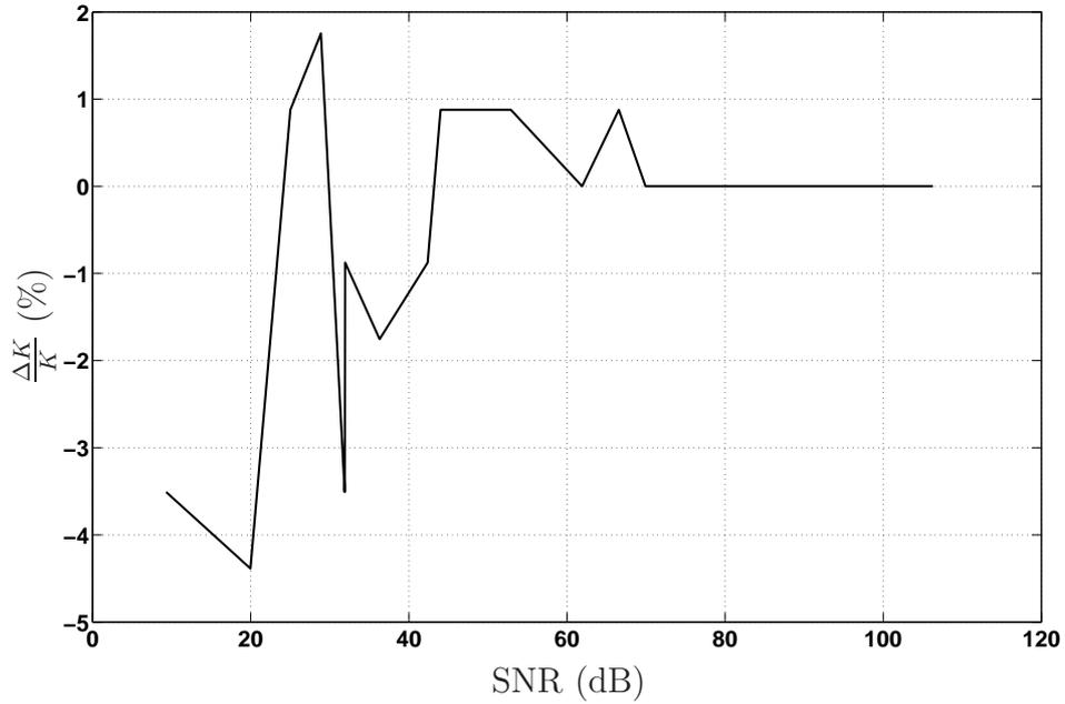
Figure 6: Enumeration accuracy as a function of the signal-to-noise ratio.
