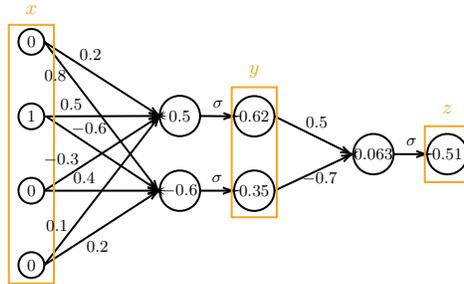
**Fig. 3.** Example of a one-hidden-layer network with computations.
