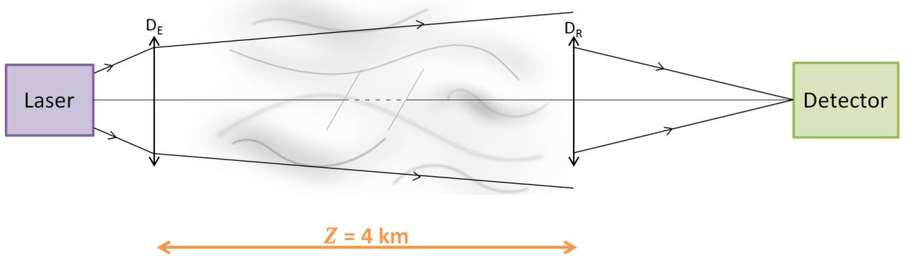
Figure 1. System architecture
